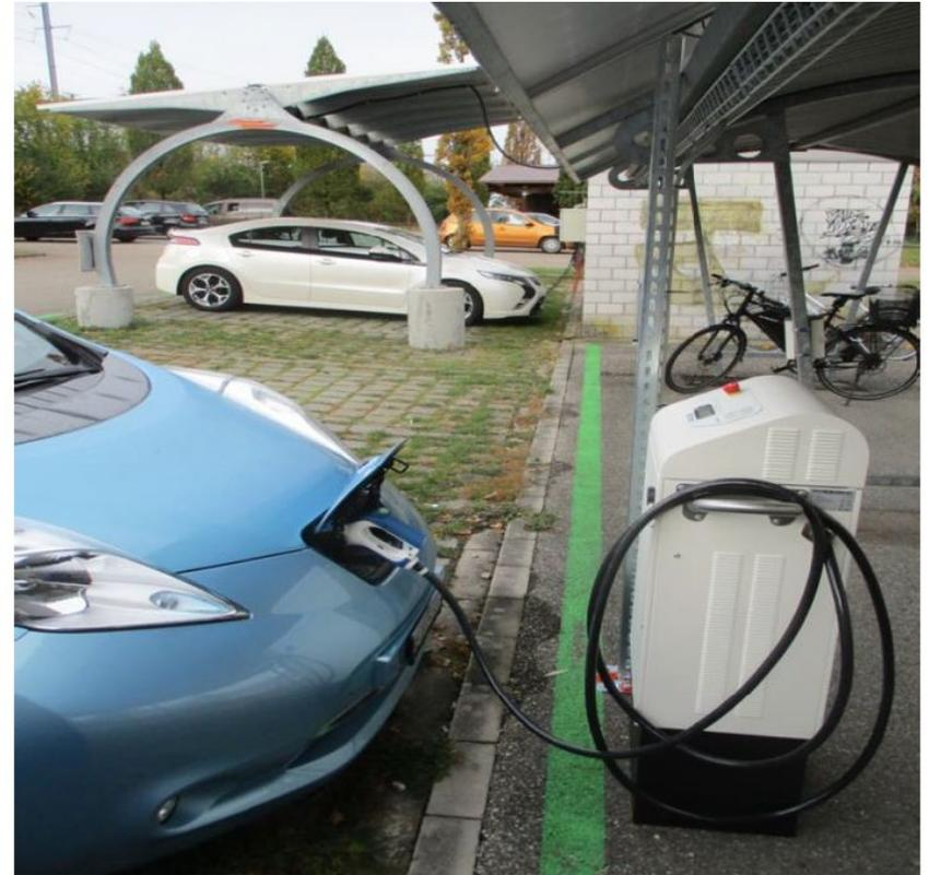
Figure 13: EVTEC bidirectional charging unit with Nissan LEAF.
